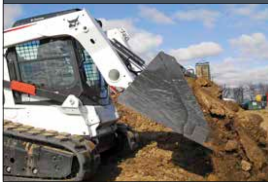
Construction/Industrial Buckets (CI): Have predrilled holes to accept bolt-on cutting edge or bolt-on teeth.
