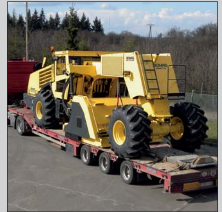
Simple transport of machine with height adjustable operator's station.
