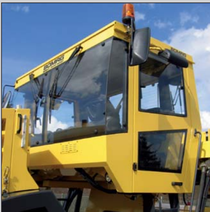
Operator's station and cab with integrated ROPS/FOPS.
