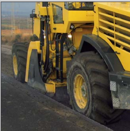
Milling close to the edge is possible on either side.
