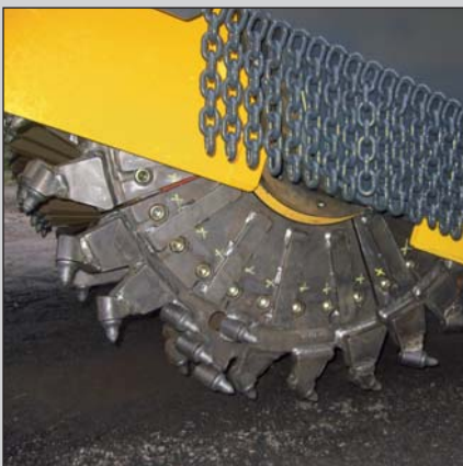
Universal rotor with individually replaceable segments.
