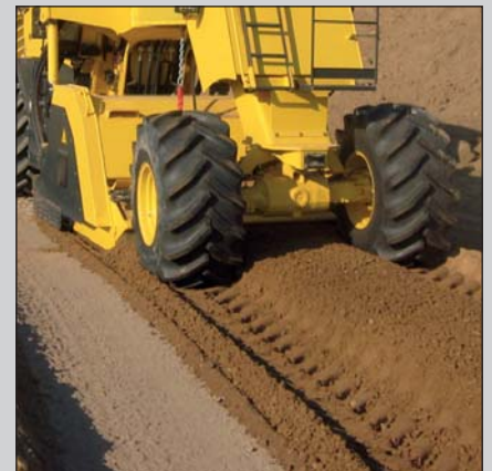
Matching of rotor speed under load ensures optimal mixing quality.
